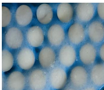
Figure 2: Starch, glycerol, and CMC mixture cast onto perforated metal plate
