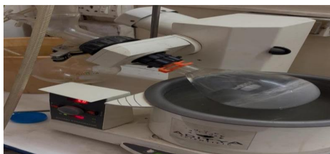
Figure 1: Rotary evaporator used in the preparation of hesperidin phytosomes
