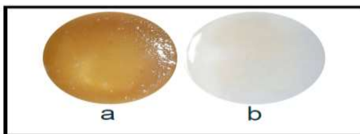
Figure 2: Silk fibroin hydrogels prepared in formulations: (a) F7 and drug loaded hydrogel in formulation of (b) F19
