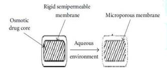
Figure 9: controlled porosity osmotic pump
