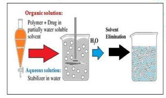
Figure 4: Schematic representation of the emulsification/solvent diffusion technique
