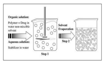
Figure 3: Schematic representation of the solventevaporation technique.
