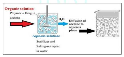
Figure 2: Schematic representation of the salting out technique
