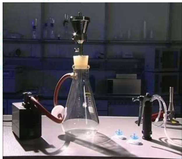
Figure 4: Direct Plate Method and Assembly of Membrane Filtration
