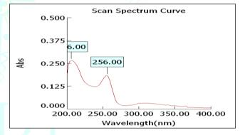
Figure 1 Determination of  $\lambda_{max}$  of PCZ
