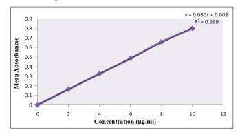
Figure 2 Calibration curve of PCZ at 256 nm
