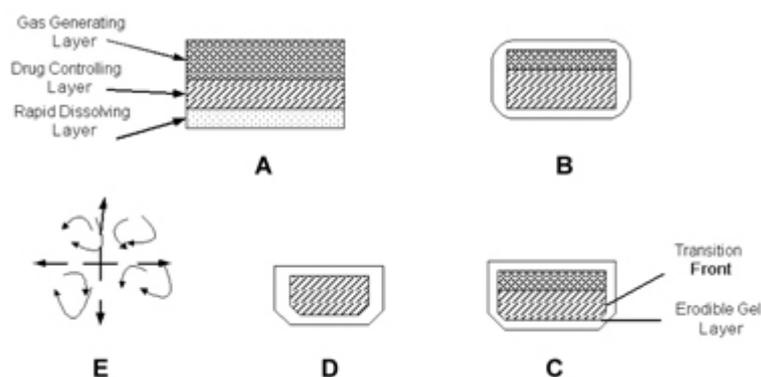
Figure 1.2. Schematic presentation of working of a triple-layer system. (A) Initial configuration of triple-layer tablet. (B) On contact with the dissolution medium the bismuth layer rapidly dissolves and matrix starts swelling. (C) Tablet swells and erodes. (D) and (E) Tablet erodes completely.
