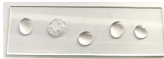
Figure 2. Catalase test. S. agalactiae was negative to catalase test as indicated by drops of hydrogen peroxide without the formation of bubbles. Drop with bubbles was inoculated with a known bacterium which is positive to catalase test.
